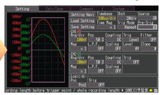
The help text crawls along the bottom of the screen, describing the function of the setting at the blinking cursor. The enhanced "Waveform Monitor" window with level meter display facilitates changes to settings by simultaneously displaying real-time input waveforms.
